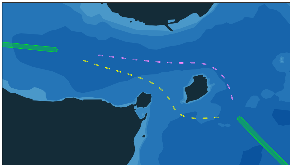
Figure 6.13: Path following simulation example, based on a simple line-of-sight guidance controller.
