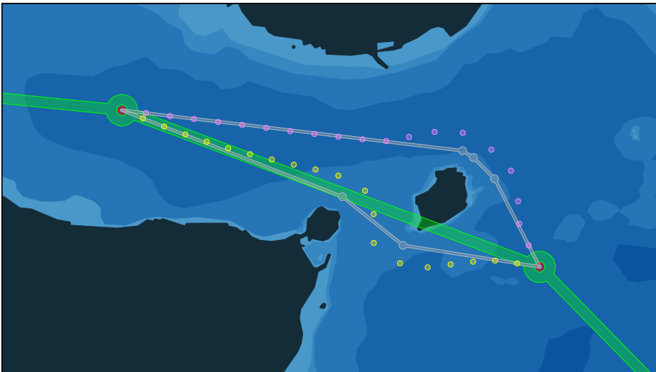
Figure 6.10: PSO demonstration of 2D waypoints along the ship route.
