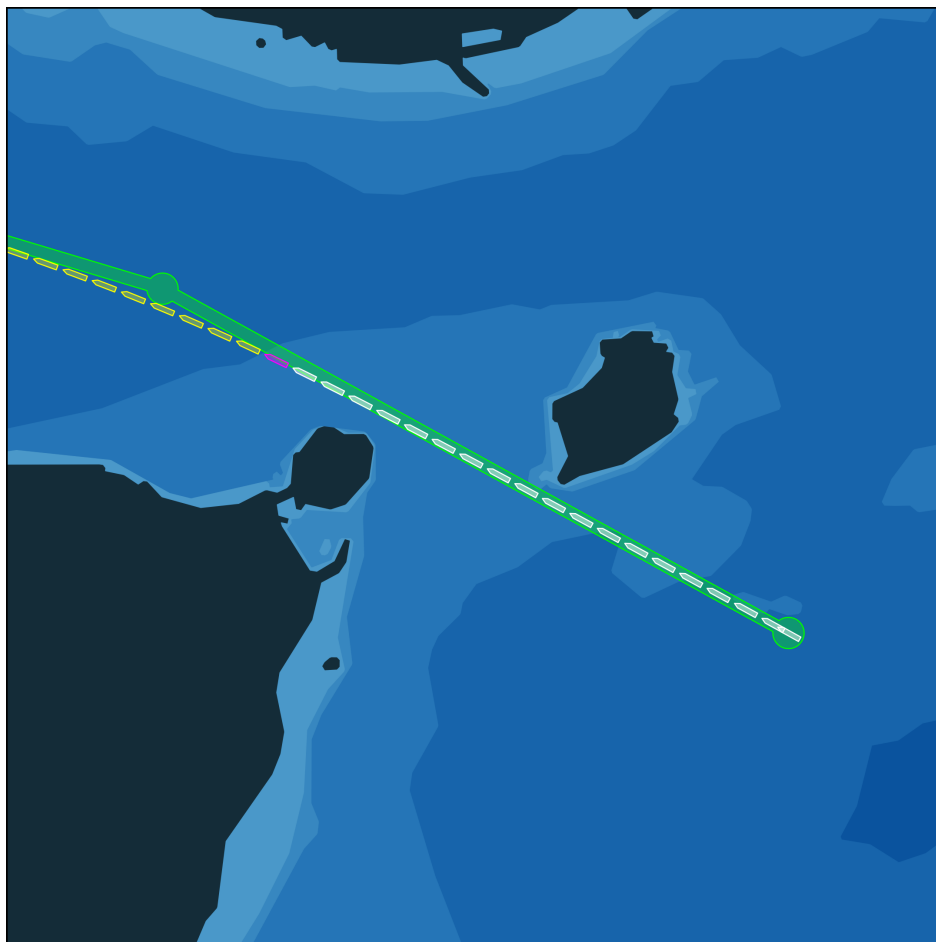
Figure 4.3: A demonstrative path following simulation using MPC, not including any risk cost terms in the cost function.
