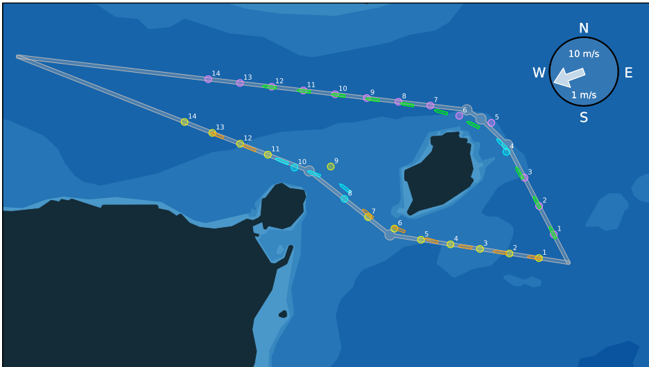
Figure 6.16: The resulting route trajectories using the complete cost function with TTG predictions.
