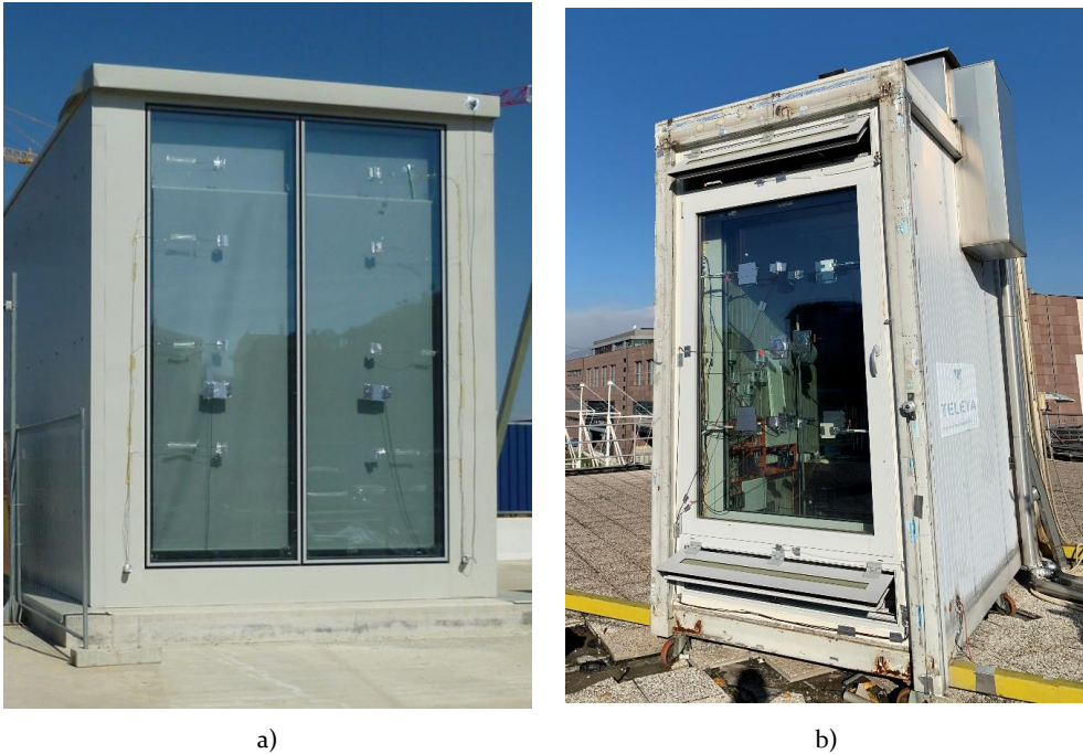
Figure 5 Test-cell facilities used in the experimental campaign. a) Mechanically ventilated exhaust DSF used in P2 and P3; b) flexible DSF used in P4 and P5.
