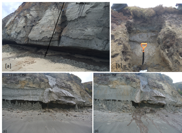
Figure 12. [a] Status of Profile#11 during the 2015 measurement. The coastal profile#11 is shown as a black line. A wave-cut niche is visible at the base of the bluffs. Image source: SAMCoT Report, 2015. [b] Permafrost inside the bluff was excavated during the field investigation in 2015. Image source: Gorshkov, SAMCoT Report 2015, [c,d] six-hour time-lapse of thermodenudation in S#1. Niche is visible at the base of the bluffs, but the bluffs are stable. Accumulation of slumped sediments at the base. Image source: Vladislav Isaev. SAMCoT Report, 2015.
