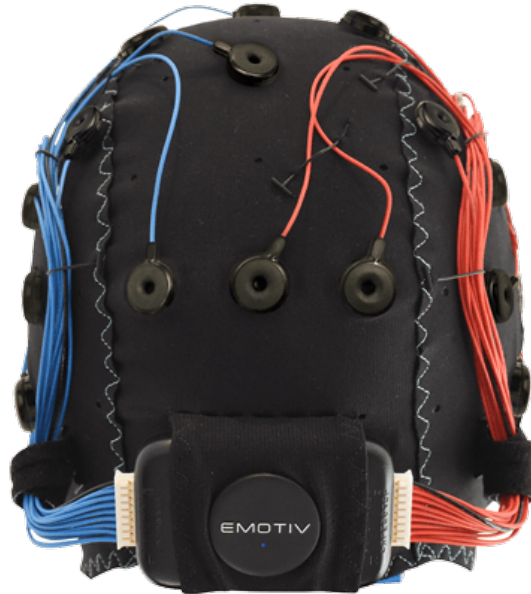
Figure 2.4: 32 channel Emotive EEG EPOC flex.
