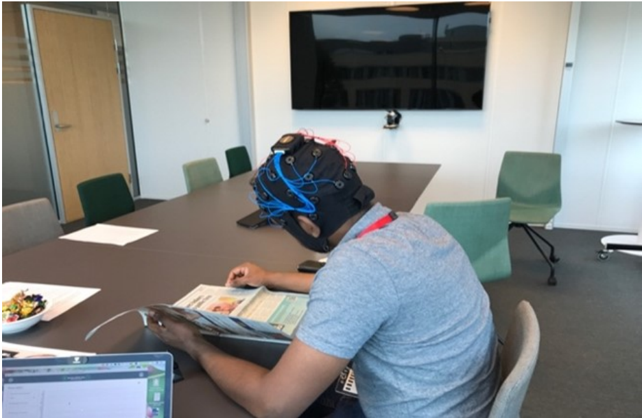
Figure C .1: A participant reading a book in a calm and quiet environment to establish baseline EEG brain activity.
