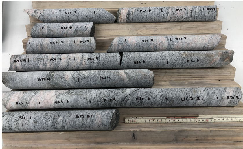
Figure 7.2: Selected rock specimens from drill core KK606KBH.
