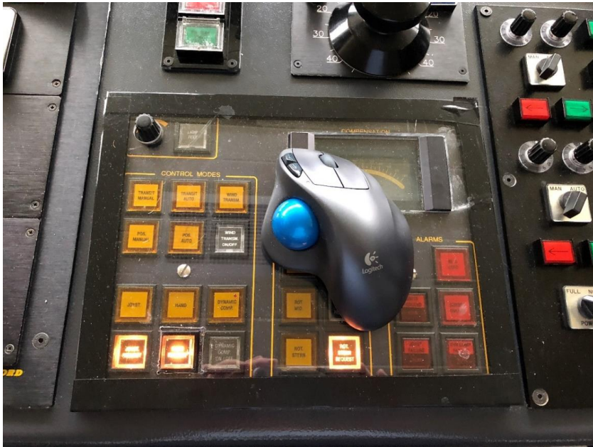
Picture 5. Example of 'adaptation of design'. A plexiglass plate is covering non-functioning buttons and a hole is carved out above the one button that is functioning. At the same time, the plate functions as a mouse mat. Photo: Brit-Eli Danielsen.
