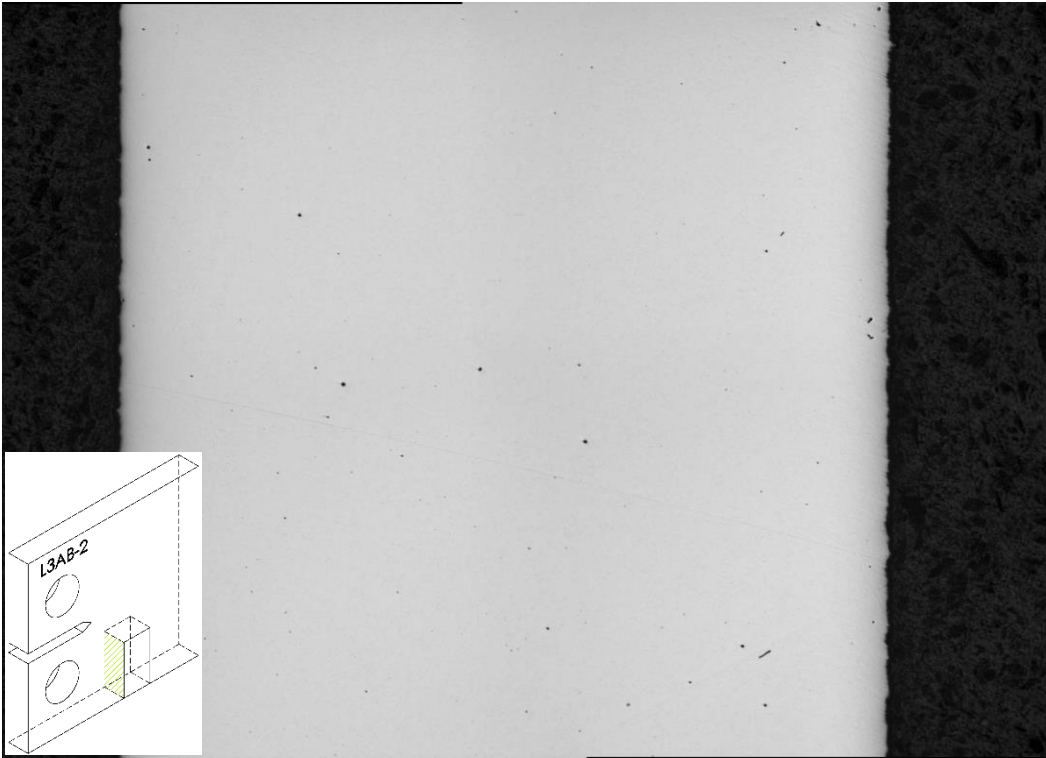
Figure 63: Overview of the incidence of defects in through-thickness sample of L3AB-2 specimen.
