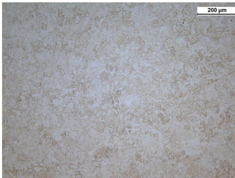
Figure 56: Microstructure of the L3MC-2 front sample at the optical microscope after chemical etching.
