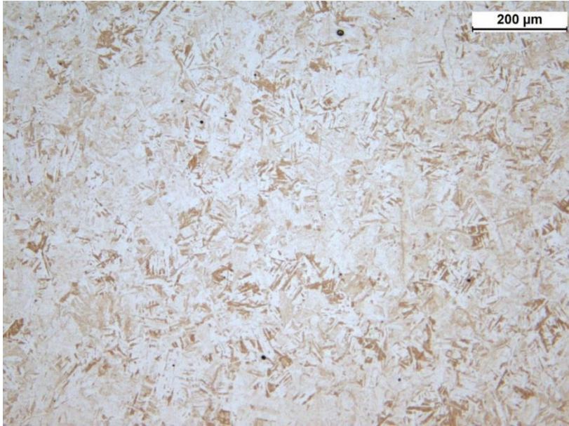
Figure 66: Microstructure of the L3AB-2 through-thickness sample at the optical microscope after chemical etching.
