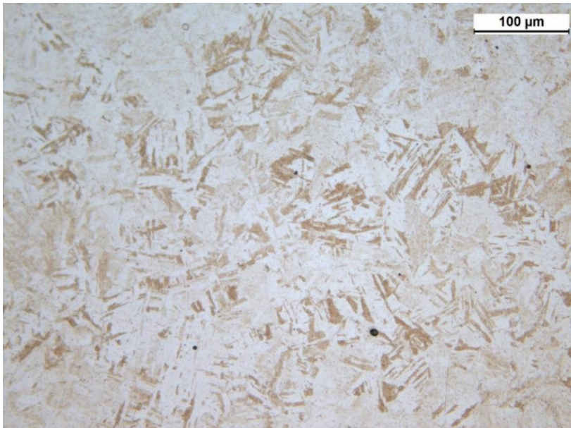
Figure 67: Detail of the L3AB-2 through-thickness sample microstructure.
