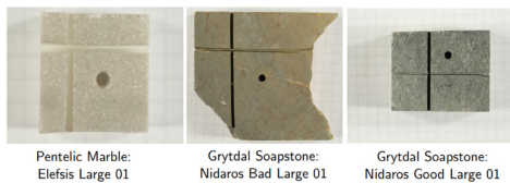
Fig. 10. Some of the stone slabs used in PRESIOUS accelerated erosion experiments [16]. The stones named Elefsis consist of pentelic marble, while stones names Nidaros consist of grytdal soapstone, representing the material of two monuments that were considered in the PRESIOUS project, the Demeter Sanctuary in Elefsis (Greece) and the Nidaros Cathedral in Trondheim (Norway) respectively.
