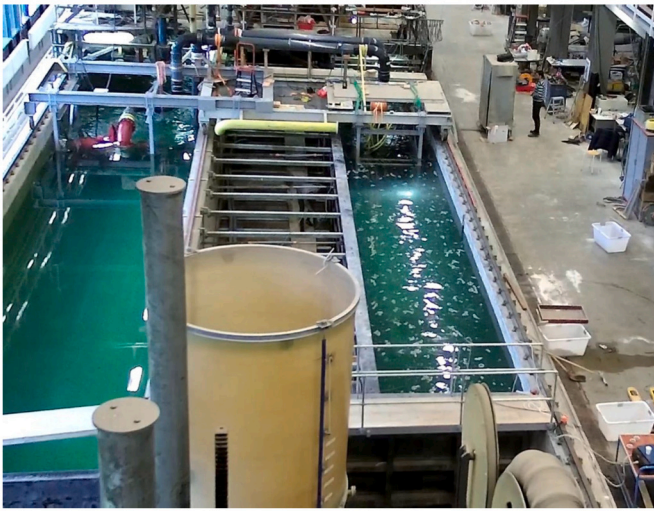
Fig. 14. Top view of the experimental setup showing the pump flume (left one) and the testing flume (right one).
