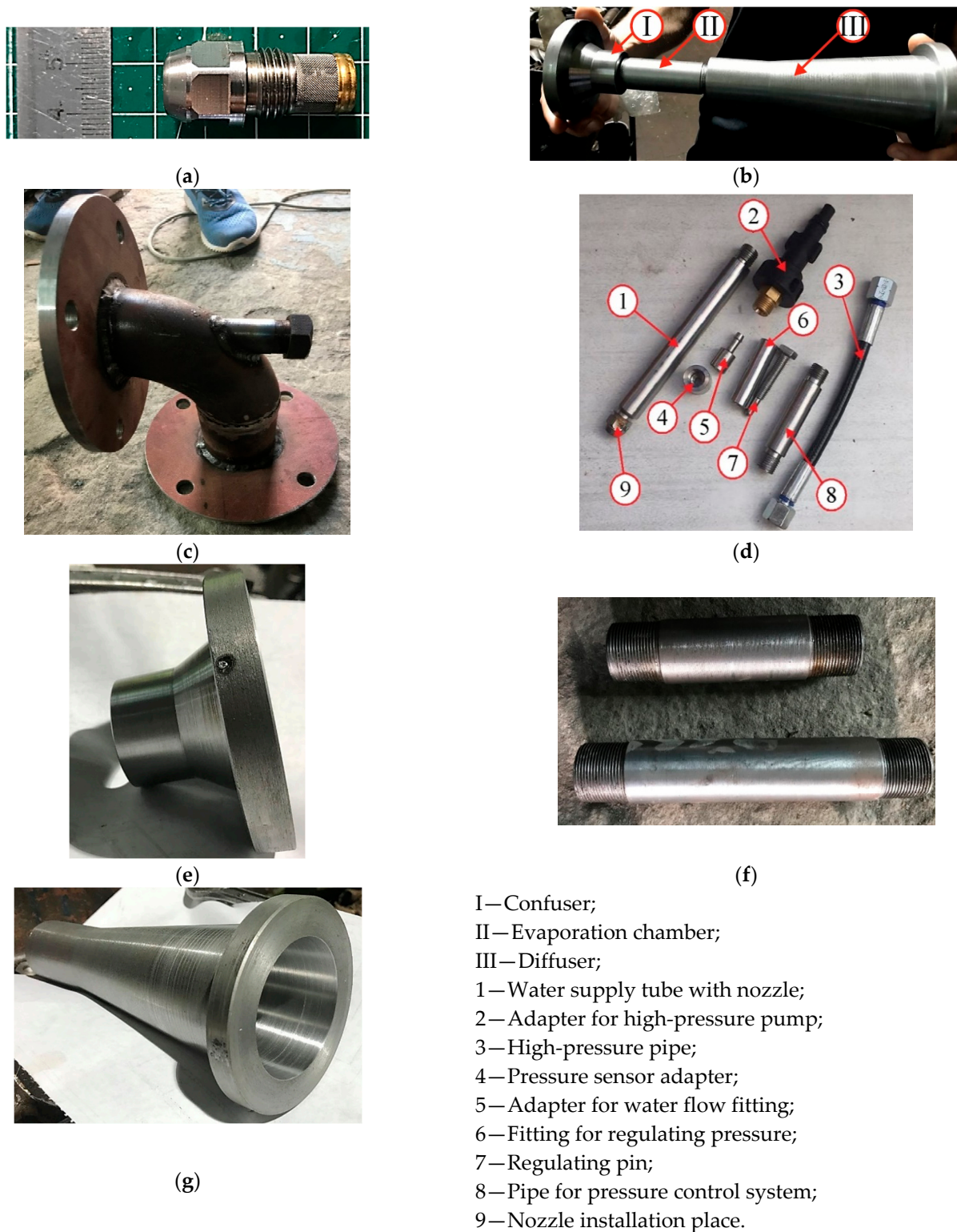
Figure 3. Experimental thermopressor: nozzle for liquid injection system (a); main elements of the thermopressor (b); receiving chamber (c); liquid injection system (d); confuser (e); evaporation chamber (f); diffuser (g).
