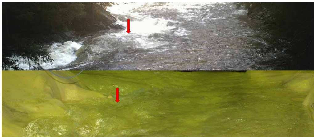
Figure 5 | Flow at \sim 200 \text{ m}^3/\text{s} in the field (top) and the hydraulic scale model (bottom). The arrows indicate the location of point GS. Flow direction from the top towards the bottom.
