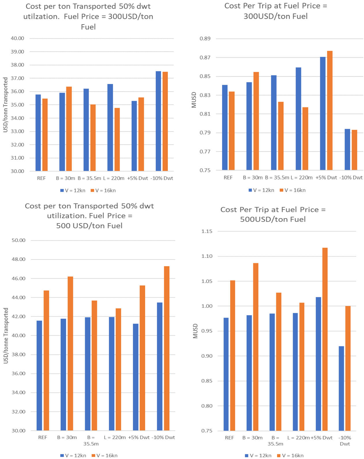
Fig. 13: Cost per ton transported and per trip at fuel price equal to 300 USD/ton and 500 USD/ton
