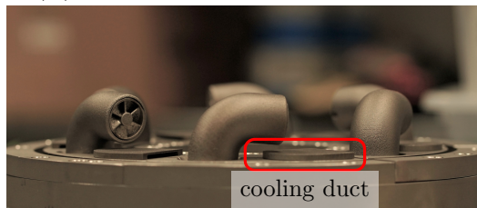
Stage (iv): cooling ducts affixed onto the top pieces.
