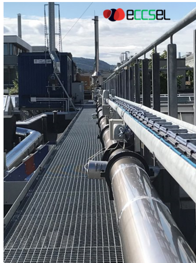
Figure 1.2.: The pipe used for experiments at the roof of SINTEF Energy Research's laboratory. Credit: SINTEF Energy Research
