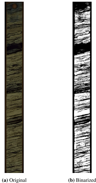
Figure 3.14: Examples of (a) an original core UV photograph; and (b) a binarized core UV photograph from well 7220/7-3 S.
