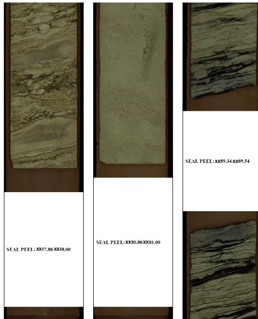
Figure 3.12: An example of a core photograph with seal peel interval from well 7220/7-3 S. The interval contains no core image; therefore, a net pay fraction label cannot be generated from that interval.
