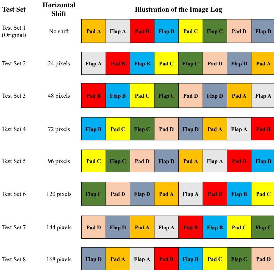
Figure 3.18: An illustration on how the test sets with horizontal variation were generated.
