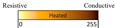
Figure 2.7: An example of an image log color scale with values between 0 and 255. The scale assigns a heated color map on the values which range from white, to orange and brown, to black.
