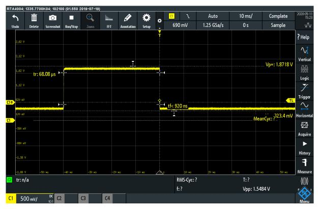
Figure 5.8: Oscilloscope reading of flash signal from HSI camera.
