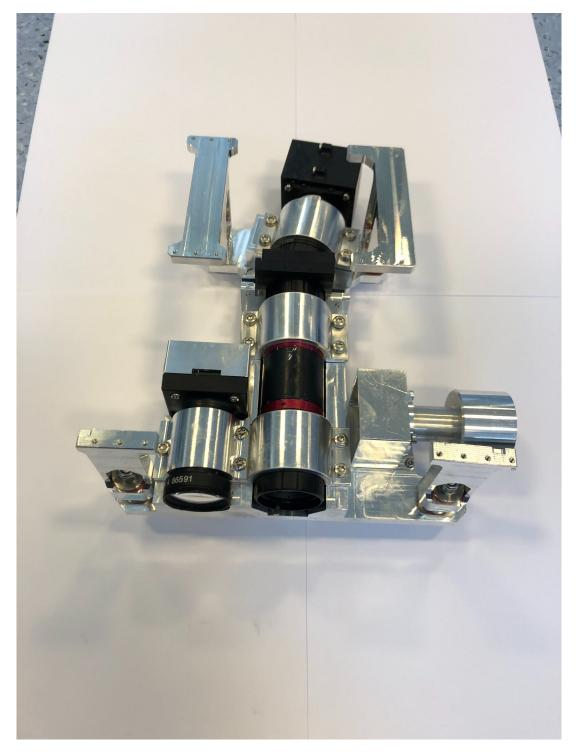
**Figure 3.6:** The hyperspectral imager (center) and RGB camera (left) mounted on platform for satellite integration. Courtesy of Martine Hjertenæs.
