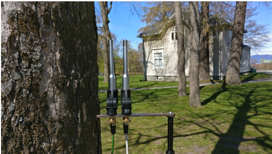
Fig. 3.8.: The microphone configuration in the bark measurement
