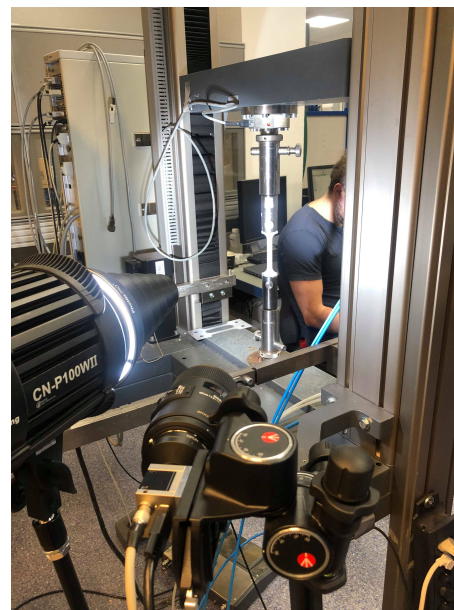
(b) Experimental set up of the tensile tests.
