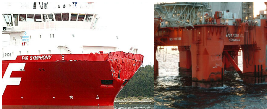
Figure 1.1: Damage on Far Symphony to the left, and West Venture to the right after collision in 2005. Picture from Pettersen and Soegaard (2005).
