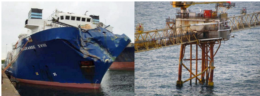
Figure 1.2: Damage on Big Orange XVIII to the left, and Ekofisk 2/4-P to the right after collision in 2009. Picture from Bjørheim (2017).
