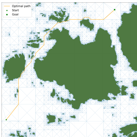
(a) Path generated using graph traversal on quadtree. ENC data courtesy of The Norwegian Mapping Authority.
