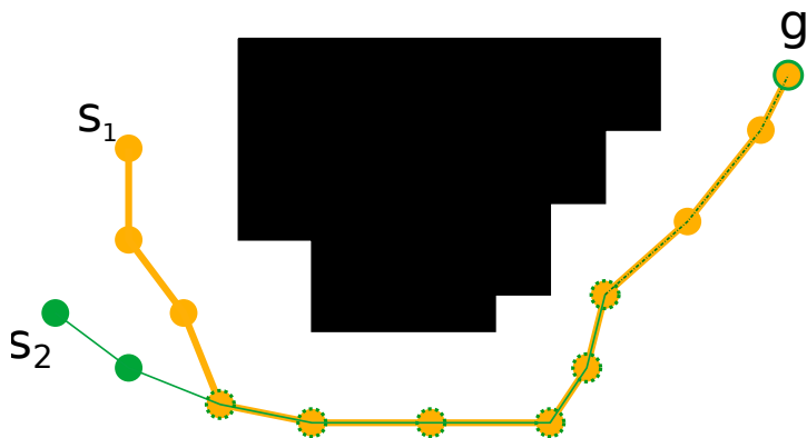
Figure 4.4: Illustration of sequence matching concept in the second query to a shortest path evaluator.
