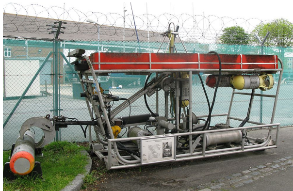
Figure 1.1: The Royal Navy ROV (Cutlet). Developed and introduced in 1950s to retrieve undetonated torpedoes and mines, [5]
