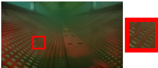
Figure 1: Motion JPEG artifacts in the Garage's sequence, showing how corners are heavily disrupted by this kind of lossy compression
