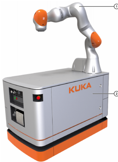
Figure 2.4.: The KMR iiwa. (1) is the LBR iiwa 14 R820 and (2) is the KMP 200 omniMove [17]
