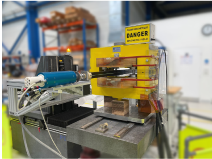
Figure 4.12: The setup of the dipole-magnet, is identical to the setup of the AirCoil-magnet, except for the magnet itself.
