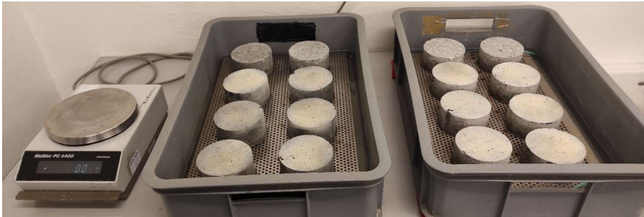
Figure 8 Capillary suction test for cracked and uncracked discs
