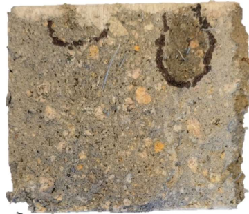
Figure 18 Water penetration front (top) for adjacent cubes sprayed with 10 % set accelerator with the water applied parallel to the direction of spraying (left) and perpendicular to the direction of spraying (right).
