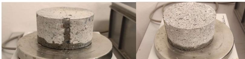
Figure 15 Left: example of capillary suction in a cracked sample. The water rise in the crack is visible compared to the lower level of capillary rise in the remainder of the specimen. Right: capillary suction in uncracked sample.
