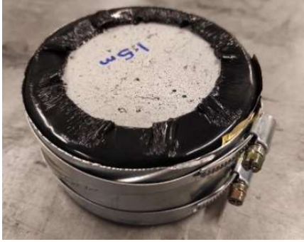
Figure 9 Cracked sprayed concrete disc wrapped in butyl tape and steel sleeve.
