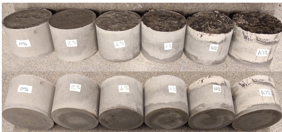
Figure 3 – Cast cylinders with different set accelerator doses
