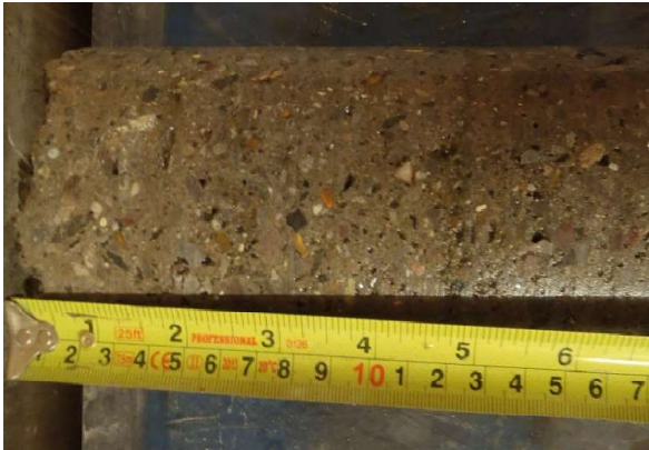
Figure 1 Example of a core from sprayed concrete lining with macro pores larger than 1 mm
