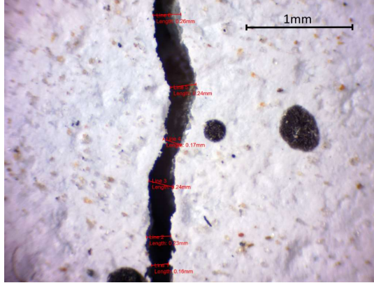
Figure 7 Example of microscope measurements of crack width for sample P11, with measurements shown in red.
