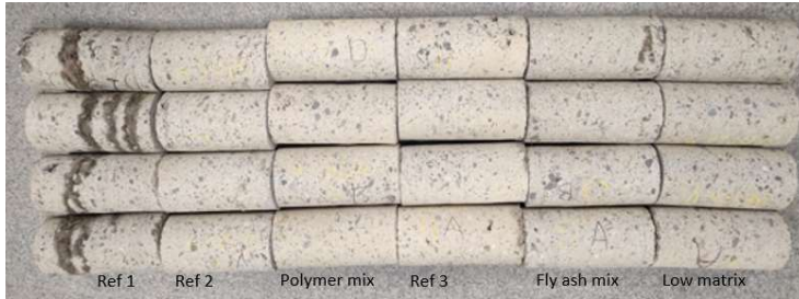
Figure 2 Identification of laminations in the cored specimens from the Drammen spraying experiments used for compressive strength tests
