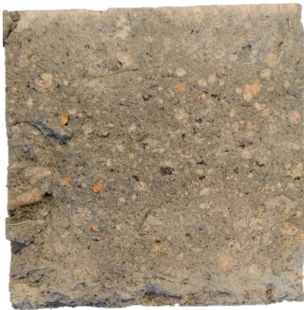
Figure 18 Water penetration front (top) for adjacent cubes sprayed with 10 % set accelerator with the water applied parallel to the direction of spraying (left) and perpendicular to the direction of spraying (right).
