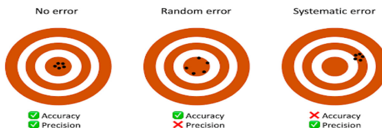
Figure 4: Illustration of the relationship between accuracy and precision and error, both random- and systematic error. Source adapted from Scribbr.com (209).
