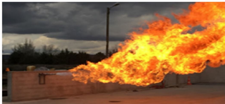
Figure 2.11: Example of a liquid hydrogen jet-fire [16].
