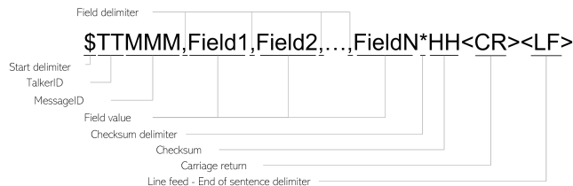
Figure 2. The format of an NMEA message.
