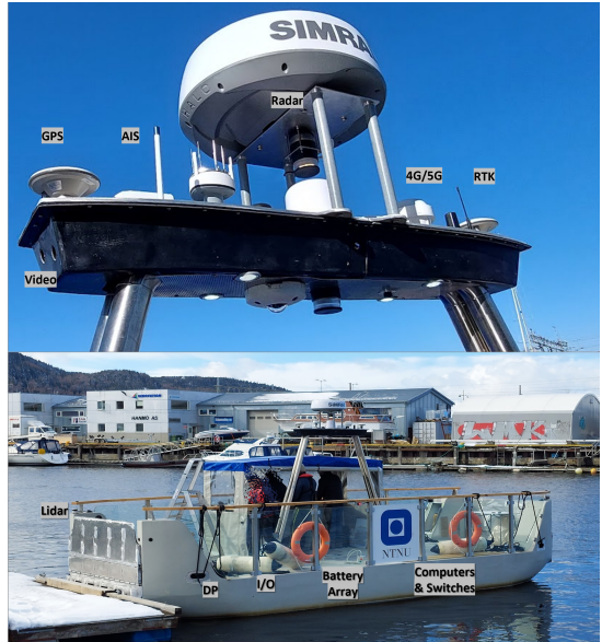
Fig. 3: The milliAmpere2 ferry with an illustration of its main cyber components
