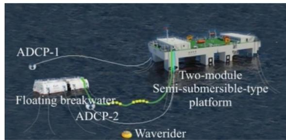
Figure 3.14: Diagrammatic sketch of the SRDP (Wu et al., 2021)
