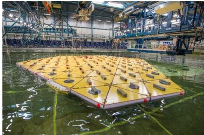
Figure 3.7: Modular floatign island basin experiments conducted at MARIN (The blue future:Horizon 2020 project Space@Sea, 2018)
