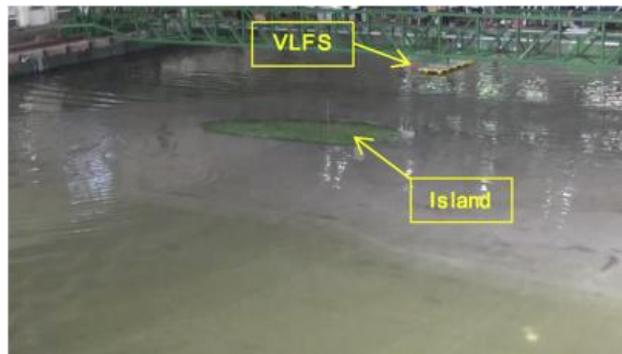
Figure 3.11: Model test of a semi-submersible VLFS in the head wave (Ding, 2015; Ding et al., 2017)
