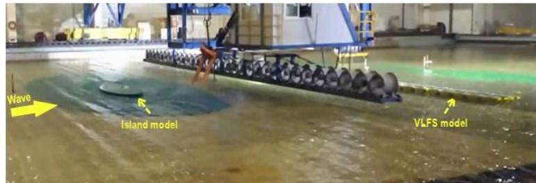
Figure 3.10: Model test of 8-module VLFS model in the basin at Shanghai Jiao Tong University (Ding et al., 2019)
