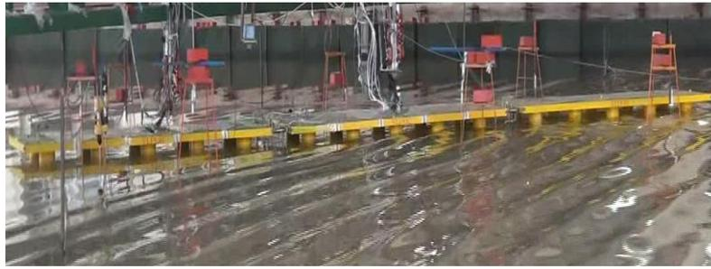
Figure 3.9: Model test of 3-module semisubmersible platform in the basin at Dalian University of Technology (Ding et al., 2017; Wu et al., 2017b)
