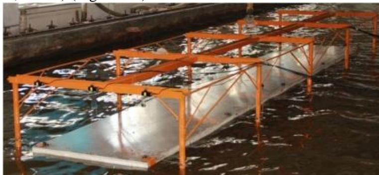
Figure 3.8: The VLFS model used in the experiment of Cheng et al. (2016a).
