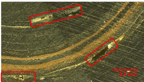
a) Small voids in Group B in the mainwall insulation. Height: 0.07 mm and width = 0.2 mm.
