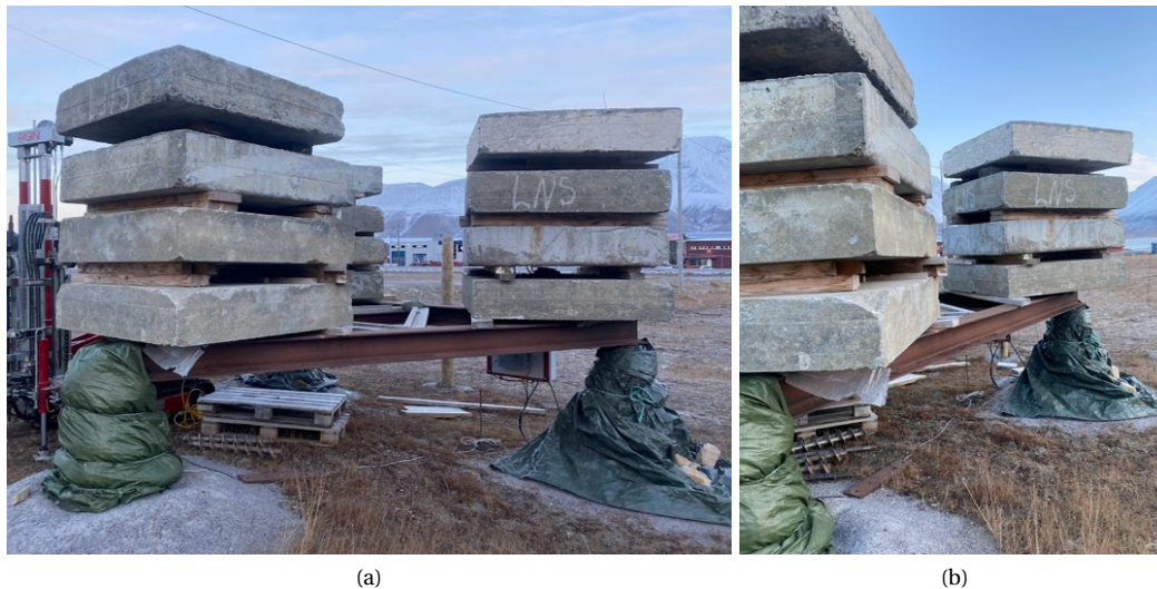
Figure 4.4: Pictures of the pile loading test after the last loading (12 concrete slabs).
