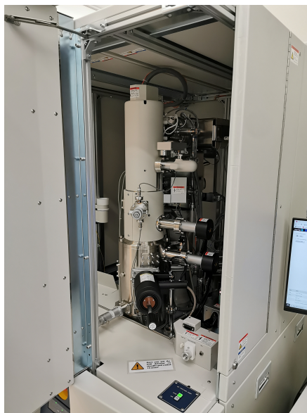
Figure 2.10: Hitachi S-5500 S(T)EM
