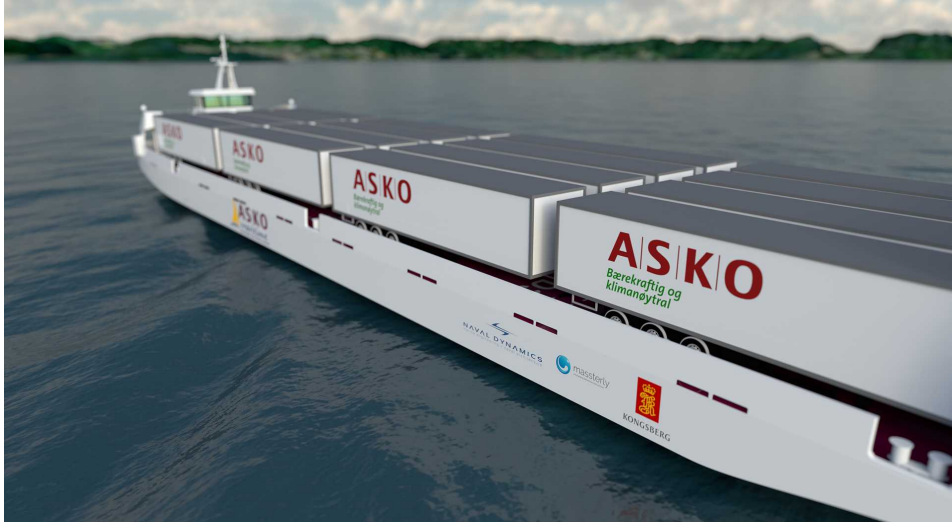
Figure 1.1: ASKO and Kongsberg Maritime have constructed two small, autonomous, and zero-emission cargo vessels capable of carrying 16 trailers across Oslofjorden in Norway. Their operation will remove 150 daily diesel truck trips from the congested roads in the Oslo area. Photo: Courtesy of Kongsberg Maritime.
