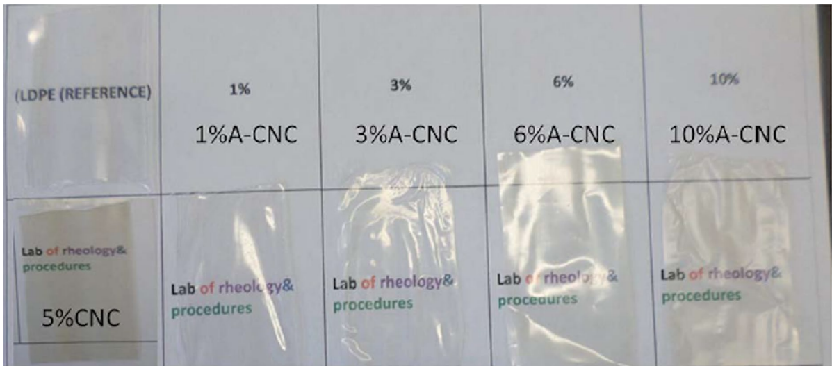
Fig. 2 Comparison of extruded polyethylene films containing CNCs and CNCs with adsorbed PEO-PPO-PEO (A-CNC). Image reproduced from Nagalakshmaiah et al. (2016)
