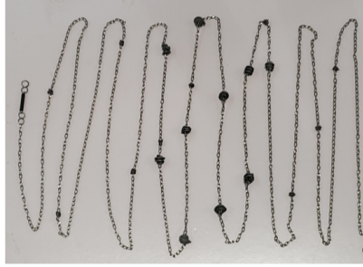
Figure 16: A produced mooring line model used in the experiment.
