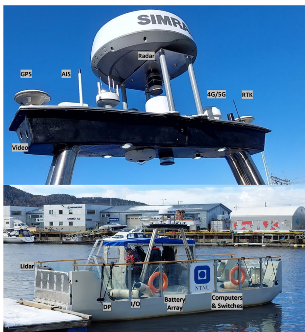
Fig. 3 MilliAmpere2 ferry with an illustration of its main cyber components
