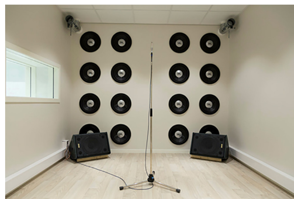
FIG. 4. (Color online) The room where the NEWT experiment is performed. The loudspeakers used for the NEWT are located on the walls to the left and right as shown in the picture. This room is usually also used to carry out standard audiometry tests.
