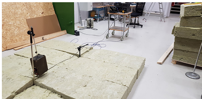
FIG. 1. (Color online) The setup is depicted for the spherical decoupling method used in laboratory exercise 3 to estimate the impedance of a sample of mineral wool from impulse-response measurements in two microphone positions successively.
