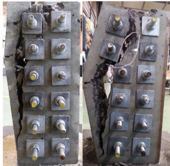
Figure 10. At ultimate failure, WSR (left), and NSR (right)
