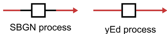
Figure 1: The SBGN process glyph versus the yEd process glyph. In black there are represented the process glyph (square box) and the ports (black line). In red there are represented the incoming and outgoing arcs. The SBGN process glyph connects to these arcs through the ports which is represented by the two black lines on each side of the square box. The representation of yEd of a process does not consider ports by default: The incoming and outgoing arcs are directly connected to the process square box.
