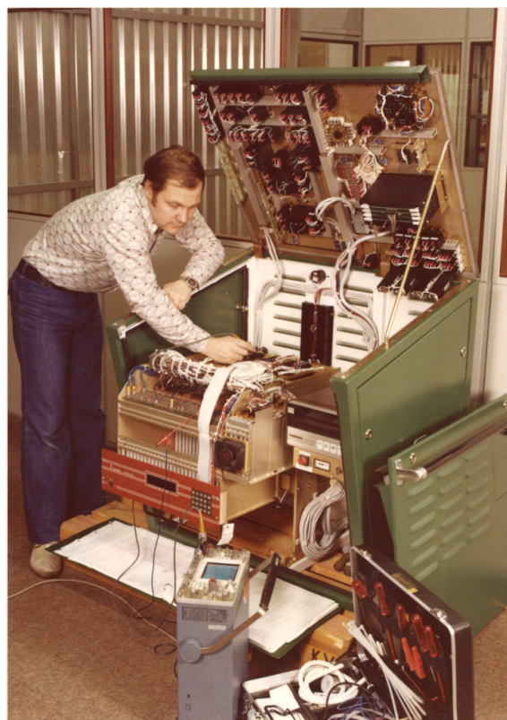
Figure 4: The ADP311 was more compact than the ADP500 series, with all electronics now collected in the console. The photo shows Odd Inge Tangen performing troubleshooting on the KS500 computer. Photo: KM.
