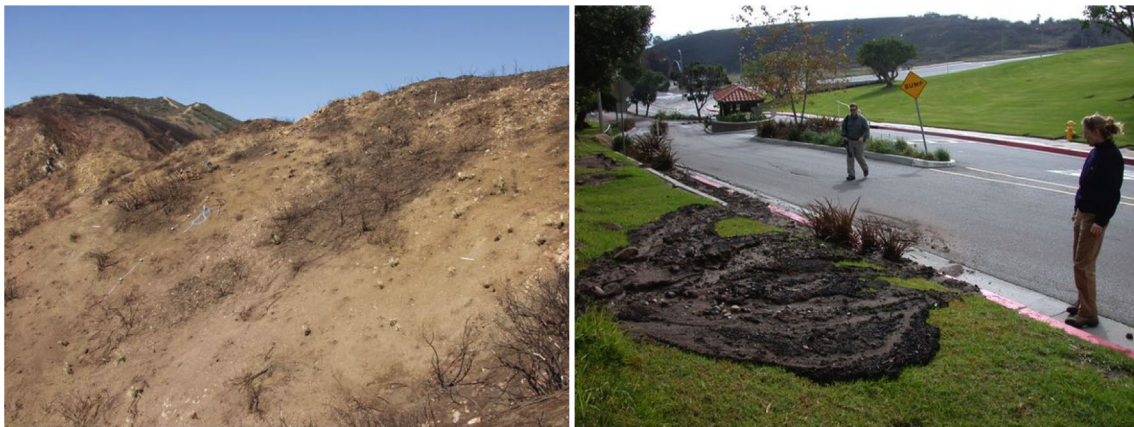
Fig. 2 Left: Photograph of a burned hillslope with rainfall, overland flow, and soil moisture monitoring instrumentation after the 2007 Canyon fire, but before rainfall, on the Pepperdine University Malibu, California campus. Right: Photograph from December 19, 2007, of a
