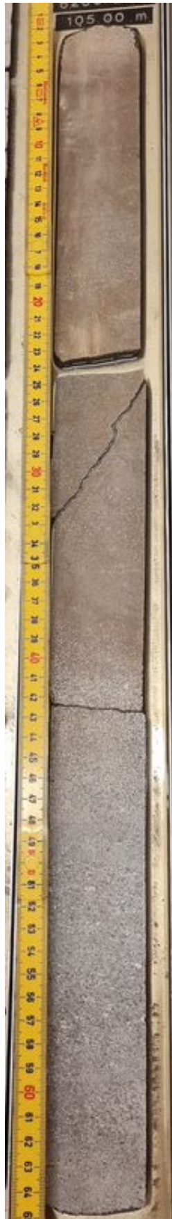
Figure 23: Core photo showing well cemented bed with increasing browning to the top, interpreted as siderite cemented bed.
