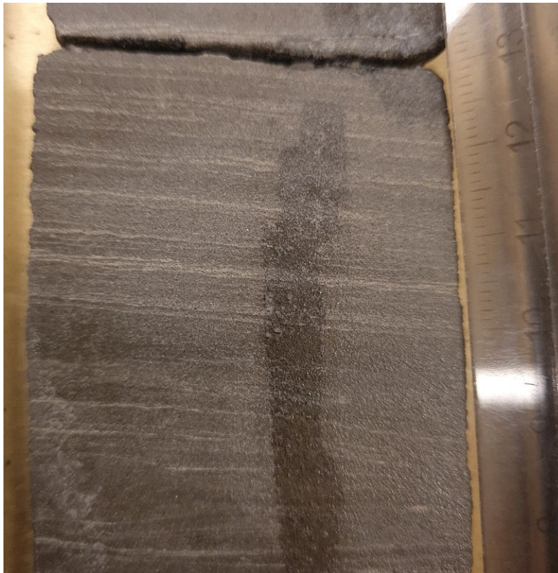
Figure 29: Core photo showing very small sandy ripples in a muddy deposit. The crack in the upper part of the photo is at depth 60.87 m. Ruler for scale.
