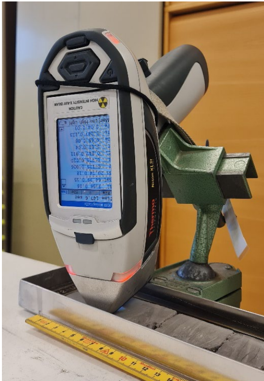
Figure 7: Setup of the pXRF during scanning of the core.
