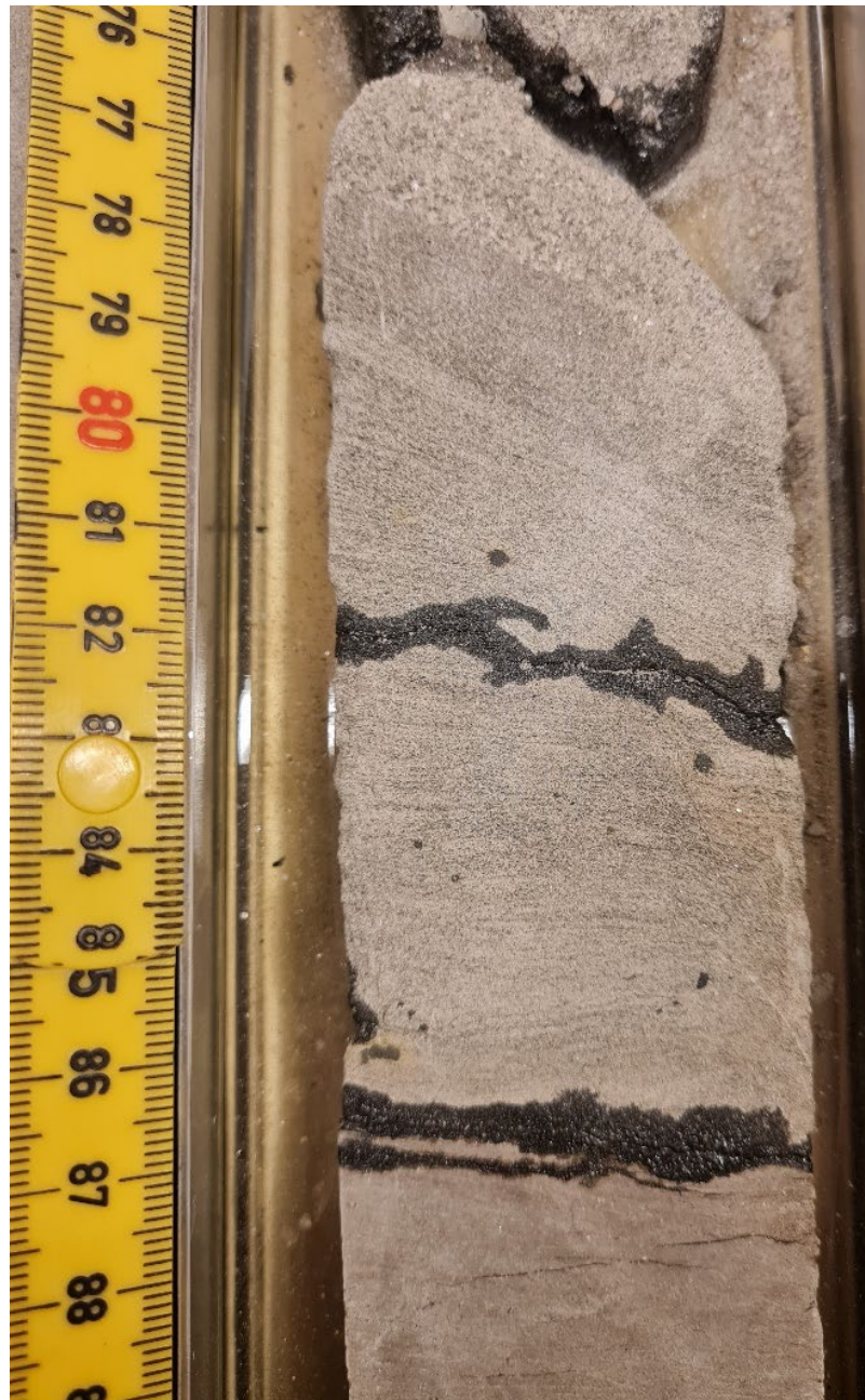
Figure 10: Core photo of hummocky cross stratification observed at depth 158.77 m. The increasing inclination on the lamination up the bed is characteristic for hummocky cross stratification.
