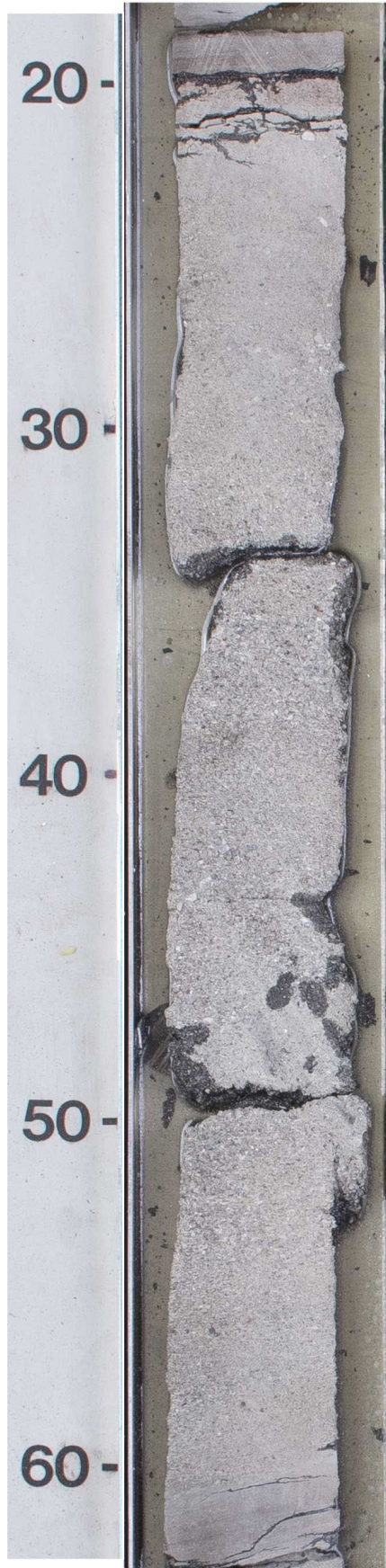
Figure 42: Core photo showing a grain flow deposit with the base of the flow at 162.60 m depth.
