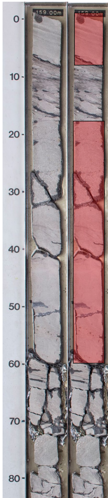
Figure 50: Core photo showing complex flow deposits, with alternating dense and dilute deposits. The dilute deposits are marked with red.
