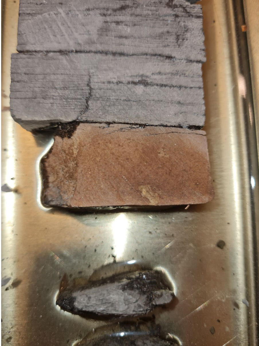
Figure 24: Core photo showing iron concretion at depth 73.81-73-83. The interval is 2 cm thick.
