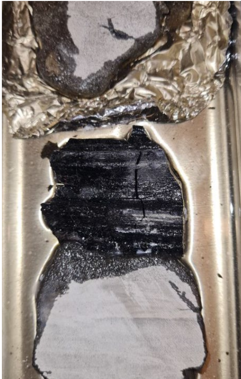
Figure 15: Core photo showing a piece of wood turned into coal. The piece of wood is 3 cm thick at depth 179.58-61 m.
