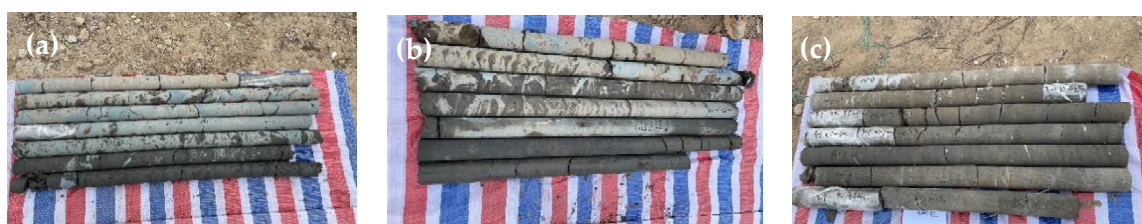
Figure 7. Influence of mixing times on the integrity of the mixing pile: (a) two times, (b) four times and (c) six times.
