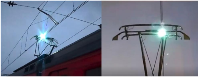
FIGURE 1 Electric spark on pantograph-catenary
