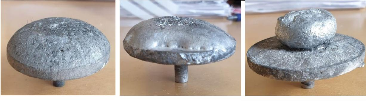
Figure 6, Deposits obtained at  $T=965^{\circ}\text{C}$  for Blank test to the left, 3 wt. % Mn initially in the bath in the center, and 1 wt. % Si to the right.
