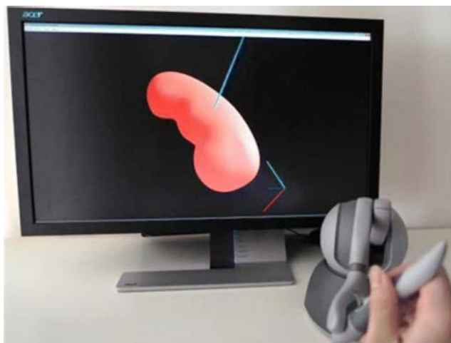
FIGURE 4. Zhang et al. [108] used cellular neural networks to model soft tissue behavior of a kidney, and interfaced the simulation with a Geomagic Touch haptic device.
