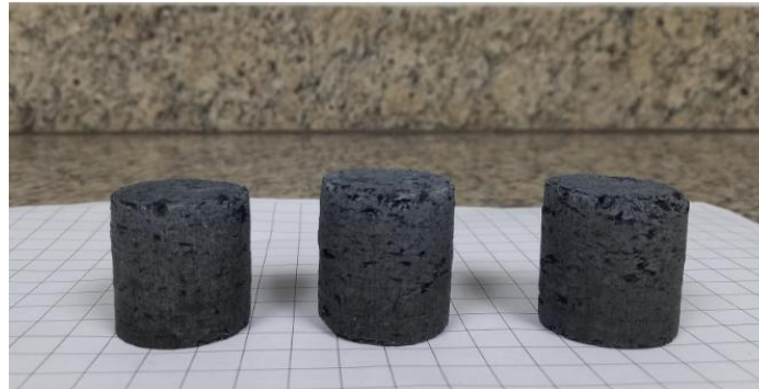
Figure 1. Self-reducing briquettes (BM12-A4) produced with sodium silicate binder.
