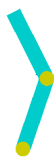
Figure 3: DoublePendulum and Acrobot: 2 link under-actuated pendulum systems fixed to a freely rotating point at the end joint and actuated at either the end joint or the middle joint. The figure is a screenshot of the system in its upright state.
