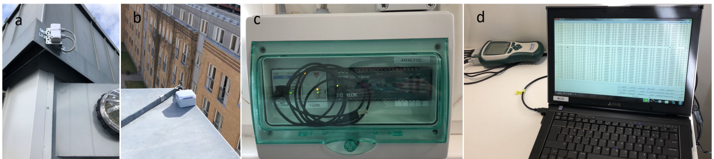
Fig. 7. Monitoring equipment: (a) Monitoring of the VI incident on the HLP, VI im; (b) monitoring of the GHI, GHI im; (c) logging of energy consumption of each luminaire; (d) logging of the indoor illuminance measurements from the five illuminance meters.
