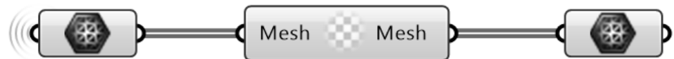
Figure 8. The component that adds a middle node on all mesh edges for quadratic finite elements.
